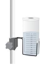
Fill the canister with water to the 0 cm line
