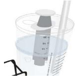
Maintain the water level to the 0 level. Water level may be adjusted by inserting a syringe through the center hole into the water for aspiration.
