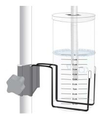
Attach the 10mm corrugated tube with air diffuser to the expiratory limb of the continuous flow breathing circuit. Insert the tube through the center hole to the desired depth with the flow rate on. Slide the tube sideways into the notch that secures the tube in position. The depth the tube is submerged in cm = positive airway pressure in cmH $_2$ O. Verify the pressure with an inline pressure gauge and adjust the depth as needed. Apply the protective cover to the top of the canister.
