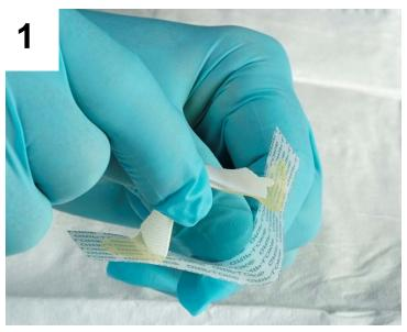
Remove the bottom release liner by holding the liner at the center and pulling straight up on the Grip-Lok from the top center.
